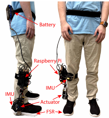
Fig. 1. Modular, backdrivable ankle exoskeleton, modified from [16]. The device can be worn unilaterally or bilaterally.
