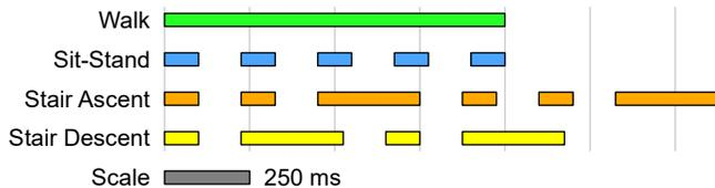
Fig. 3. The smartwatch application vibrates with unique patterns whenever the prosthesis changes activity modes. Solid lines indicate times when the smartwatch vibrations are active, and gaps indicate when they are inactive.
