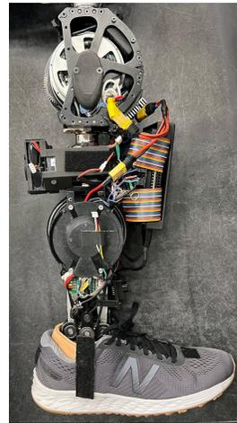
Fig. 1. The powered knee-ankle prosthesis used for this study. Users of the device can perform multiple activities: level and ramp walking, stair climbing, and sitting/standing.
