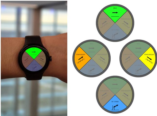
Fig. 2. Physical smartwatch (left) and user interface of the smartwatch application (right) highlighting the four available activity modes. Swiping the screen from the quadrant labeled with an activity mode to the opposite side commands the prosthesis to change into that mode.
