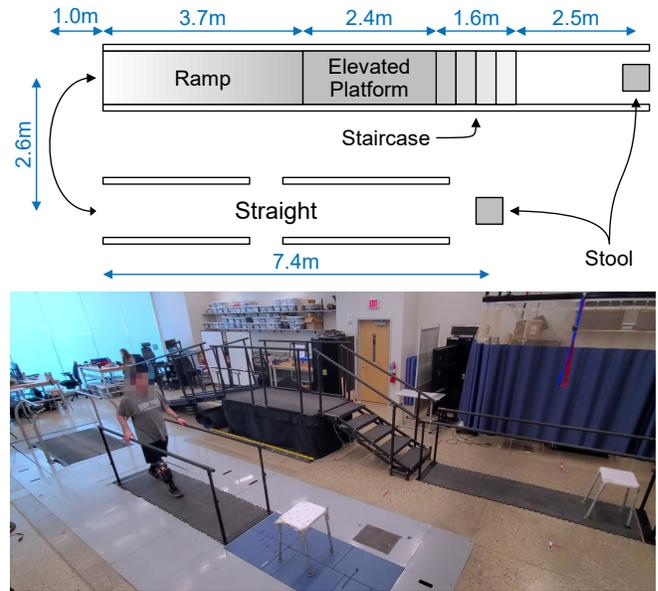
Fig. 4. Experimental setup of the multi-activity circuit, including two stools (44.5 cm seat height), a ramp (11.2° incline), and a five-step staircase (14.4 cm riser height and 33.3 cm tread depth). Top: Aerial schematic with key dimensions. Bottom: Oblique view photograph with the participant during the experiment.
